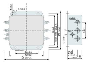
Figure 7-3 Simple Filter Outline and Installation Dimension Figure
