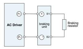
Figure 2-17 braking unit connection
