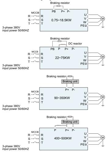
Figure 2-6 Main circuit wiring diagram
