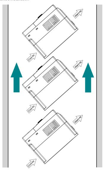
Figure 3-6 Tilt installation
