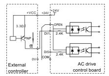
Figure 3-23 Source Wiring
