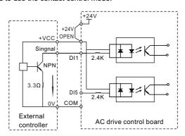
Figure 3-21 Sink wiring
