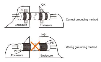
Figure 3-16 360-degree grounding technique diagram
