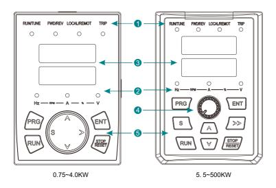
Figure 4-1 Keypad diagram
