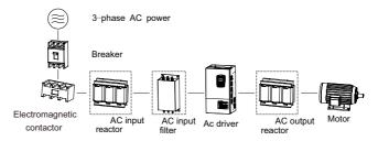
Figure7-1 EMC external fittings installation diagram
