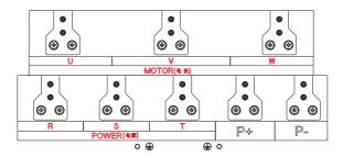
280~350KW main circuit terminal diagram
