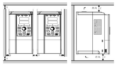
Figure 3-4 Parallel installation
