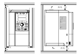
Figure 3-3 Single installation
