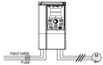
Figure 3-25 Fuse configuration diagram
