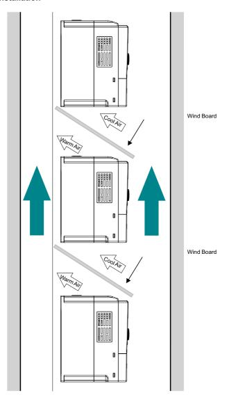
Figure 3-5 Vertical installation
