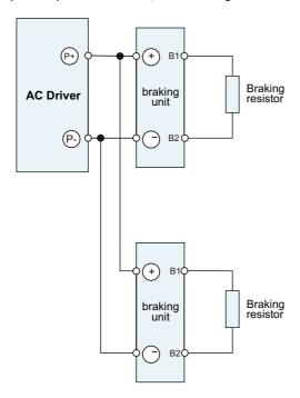
Figure 2-18 braking ones in parallel connection
