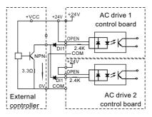
Figure 3-22 DI terminals connected in parallel in SINK mode
