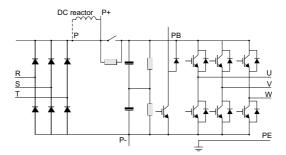
Figure 2-2 22KW~75KW Main Circuit Diagram
