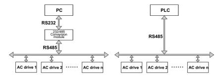
Figure 9-2 Single host/Multiple slaves networking way
