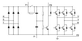
Figure 2-1 0.75KW~18.5KW Main Circuit Diagram
