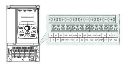
5.5~500KW Control terminal diagram
