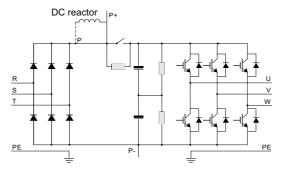
Figure 2-3 90KW~500KW Main Circuit Diagram
