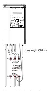
Figure 7-2 Simple filter installation diagram
