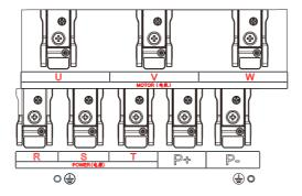
132~250kW main circuit terminal diagram
