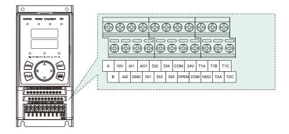
0.75~4.0KW Control terminal diagram
