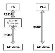
Figure 9-1 Single host/slave networking way
